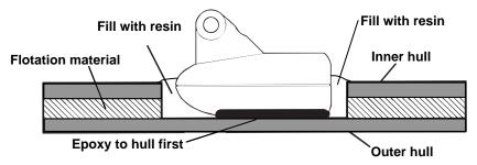
Use epoxy to place the transducer in a solid portion of the hull.
